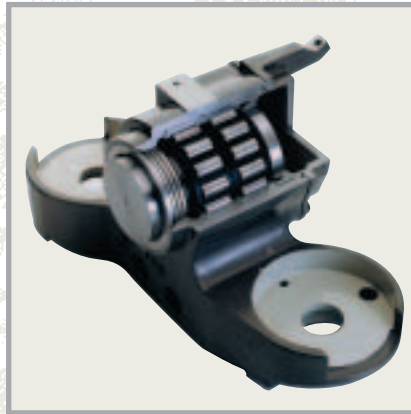
Cylindrical roller bearings with polyamide cage ET423 Metro train
