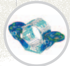
Stress analysis with BEM calculation
